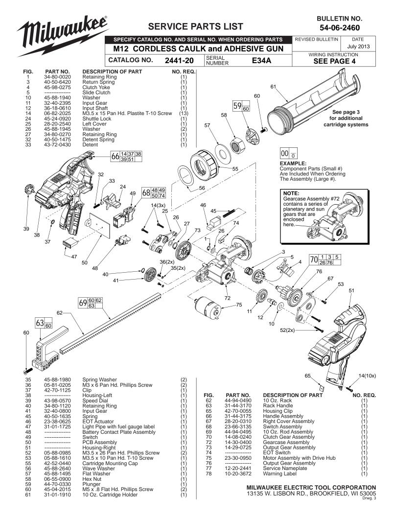
NOTE: Clutch Yoke #4 is to be the first clutch component installed and the last component removed from the gearcase assembly.
